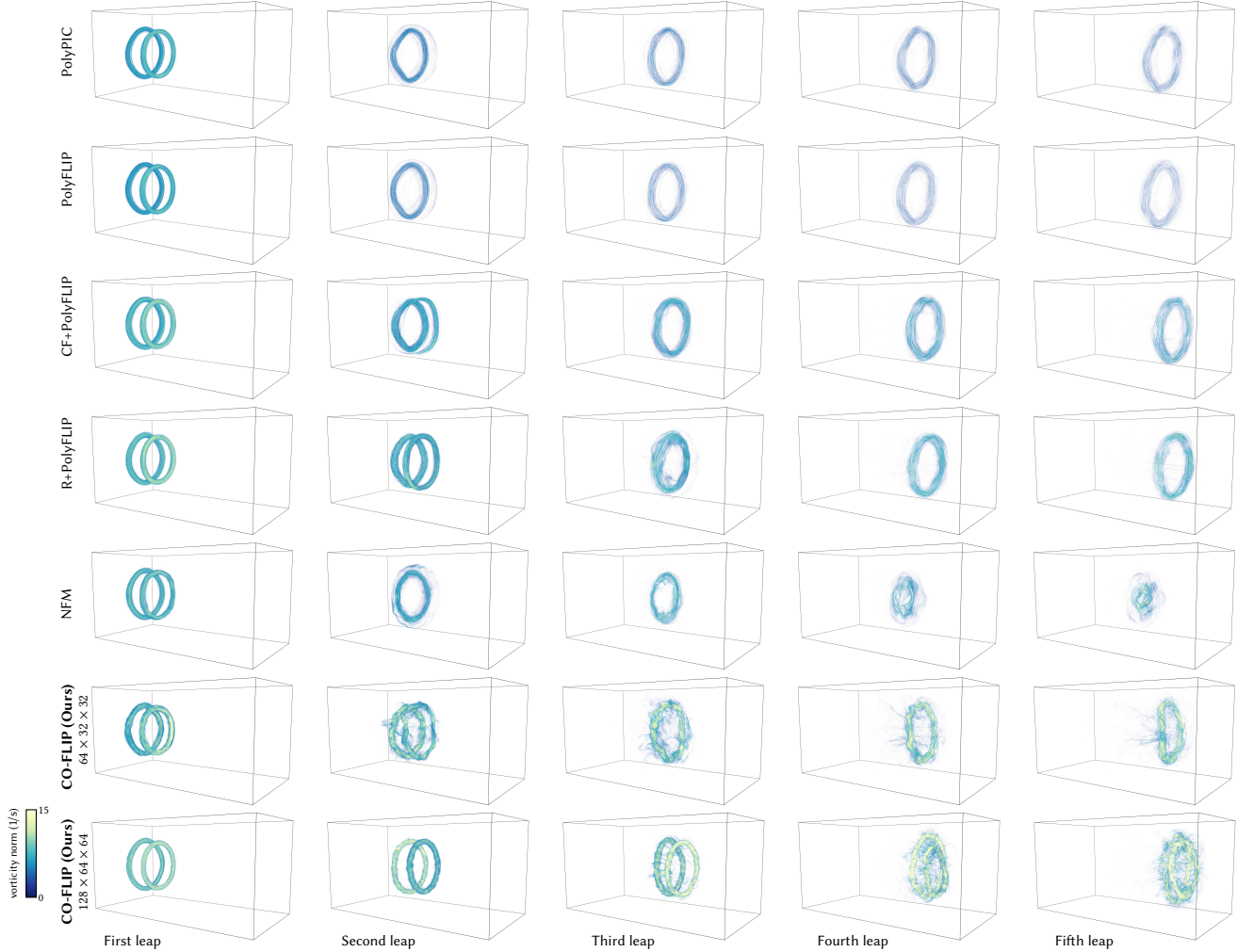
Fig. 26. Leapfrogging vortex rings in 3D. At a low resolution of 128 \times 64 \times 64 , our method (CO-FLIP) leaps five times before the vortex rings mix. At an even lower resolution of 64 \times 32 \times 32 , CO-FLIP manages to leap almost three times, which shows better behavior than some traditional works at higher resolutions. Previous methods at best (i.e. R+PolyFLIP method) leap twice.
