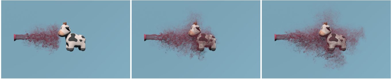
Fig. 5. A nozzle shooting out smoke and hitting a Spot-shaped [Crane et al. 2013b] obstacle. Note the intricate vortical structures our method (CO-FLIP) can create at a low resolution of 128 \times 64 \times 64 .
