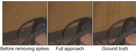
Figure 5: The image on the left shows the result of our approach before spike removal on an inset of the KITCHEN scene. In our method, we remove high magnitude spikes in the filtered image as a post-process to produce the result shown in the middle. The ground truth image is shown on the right for comparison.
