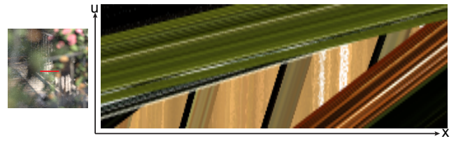
Figure 16: An xu slice through the screen-lens light field in an 8-pixel-wide region in the San Miguel scene (slice highlighted in red in the left image). The complex visibility over the lens and the samples' varying slopes prohibit sheared linear filtering.
