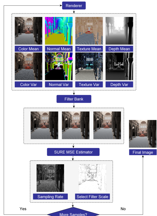
Figure 2: An overview of our algorithm, which alternates between sampling and reconstruction until reaching the sample budget. During sampling, a set of samples collects colors, normals, textures and depths over the image plane. They are used as the side information for filters in the reconstruction stage, during which, for each pixel, a set of filters are performed and the filtered value with the minimal SURE value is filled into the reconstructed image. In addition, the minimal SURE value of each pixel is recorded to guide adaptive sampling. If there are sample budgets left, more samples are shot for pixels with larger SURE errors.
