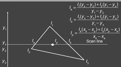
Actual implementation efficient: difference equations while scan converting
